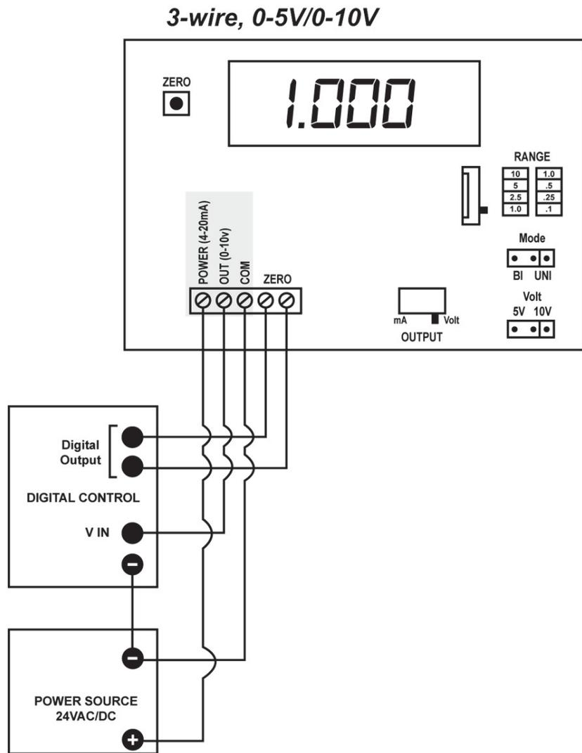
Figure 2-10 3-Wire, 0-5V/0-10V System DP Wiring
