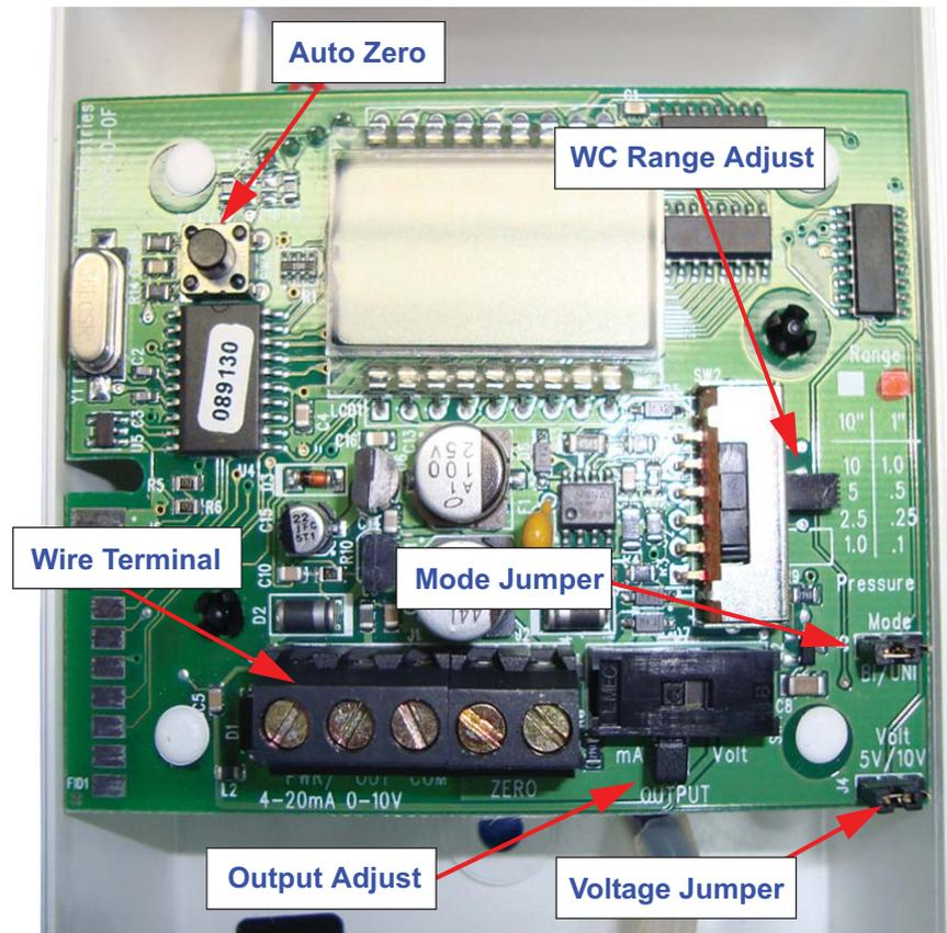
Figure 2-8 System DPS Adjustments
