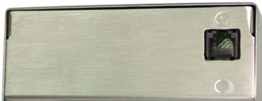
**Figure 2-5 Instrument DPS RJ-12 Connector**
