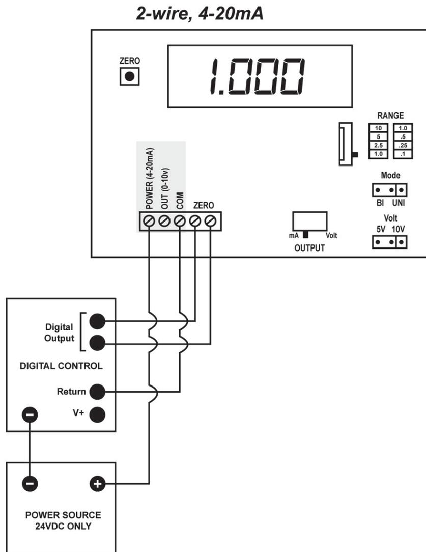
Figure 2-9 2-wire, 4-20mA System DP Wiring
