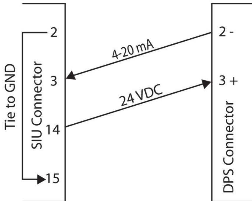
**Figure 2-4 SIU DPS: Loop Power Wiring**
