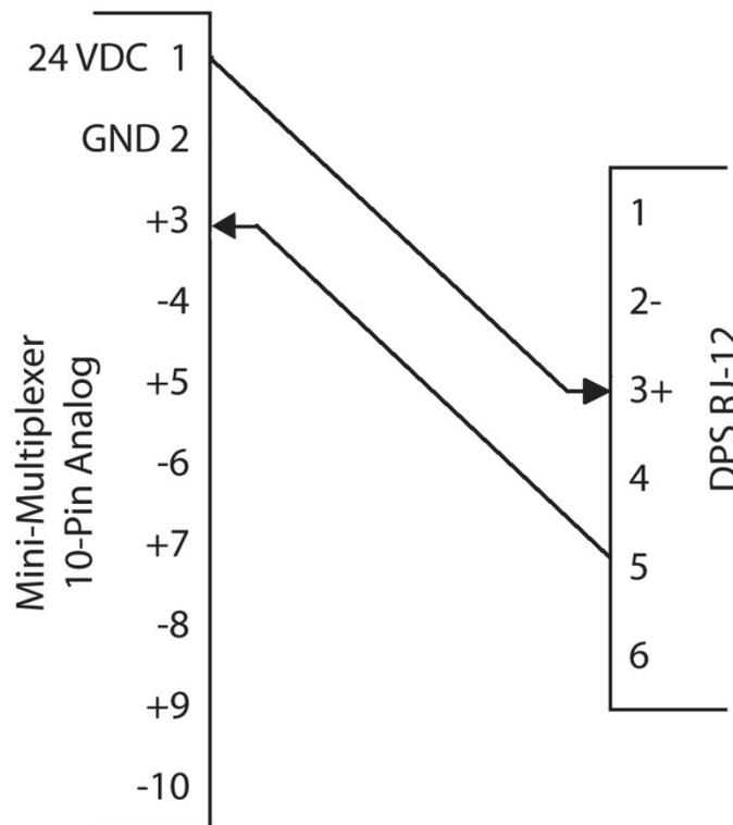
**Figure 2-7 Mini-Multiplexer to DP Sensor Wiring**
