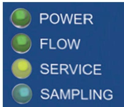
**Figure 3-1 Front Panel LEDs**
