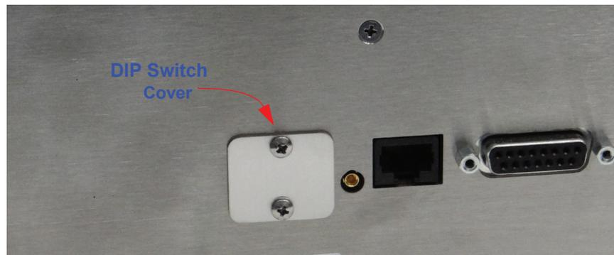
Figure 4-1 Panel Covering the DIP Switches
