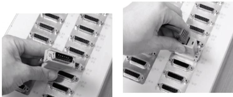
**Figure 3-6 Connecting to SIU Frequency Port**
