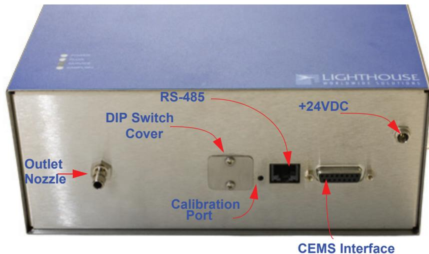
**Figure 3-4 Instrument Connections**
