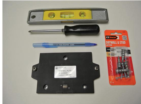
Figure 7-1 Required Tools and Hardware
