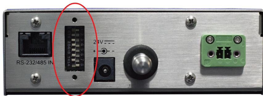
Figure 4-1 Panel Removed, Switches Exposed
