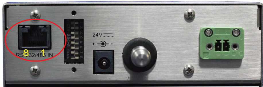
Figure 4-2 Communications Ports, Showing Pin Numbers
