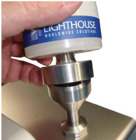
**Figure 3-10 Attach ISP Filter Cap**
