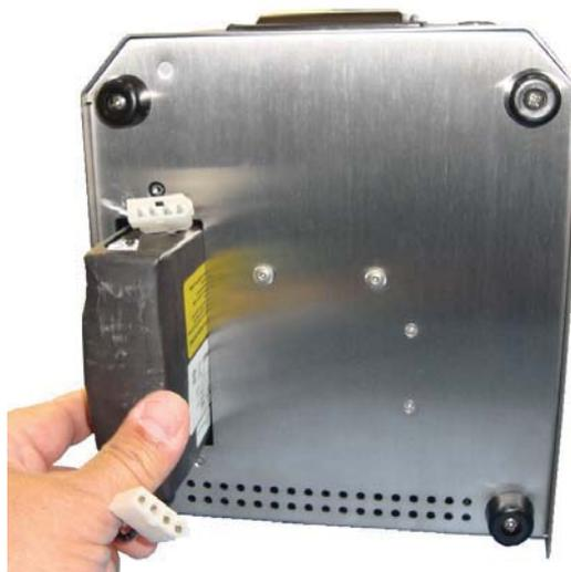
Figure 3-4 Removing the Battery
