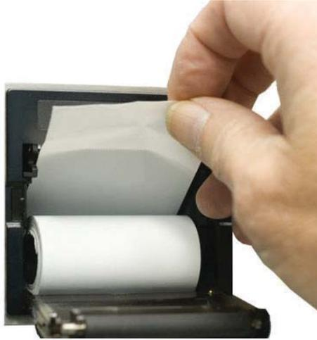
**Figure 3-13 Putting the paper into the printer**
