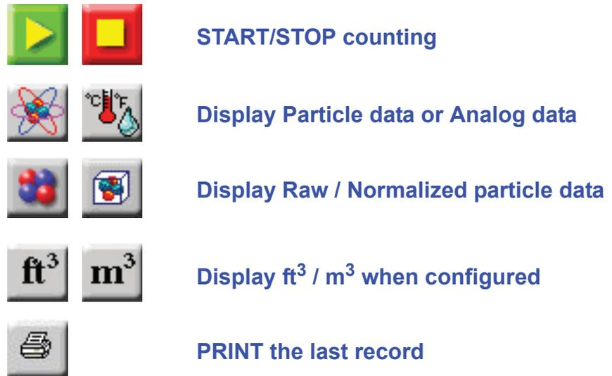
**Figure 6-12 Diff / Cuml Screen Button Actions**
