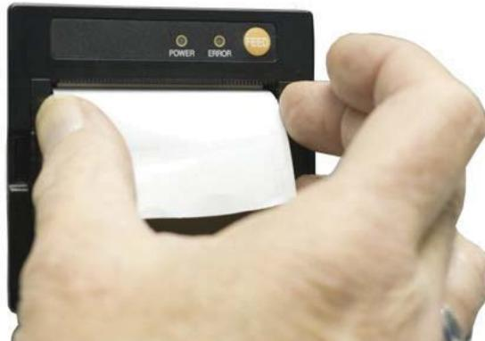
**Figure 3-14 Aligning the paper**
