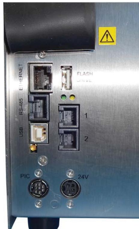
Figure 7-1 The Communications Ports
