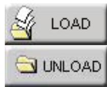
The LOAD and UNLOAD buttons add or remove the highlighted recipe as the instrument's current operating configuration.
