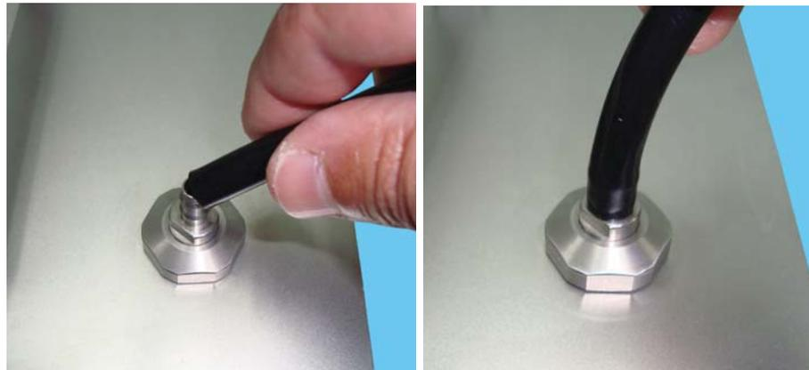
**Figure 3-6 Attaching tubing to Inlet**
