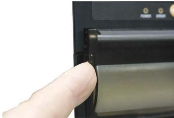
**Figure 6-58 Door is Closed and Latched**
