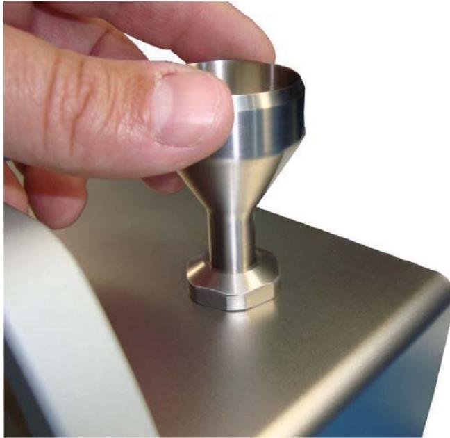
**Figure 3-9 Install ISO Probe**
