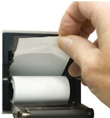
**Figure 6-59 Correct Paper Loading Position**
