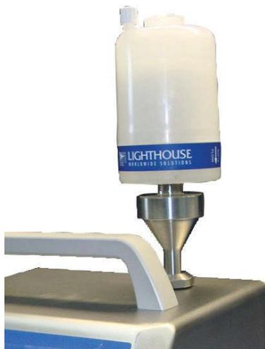
**Figure 3-11** ISP Filter Cap Installed
