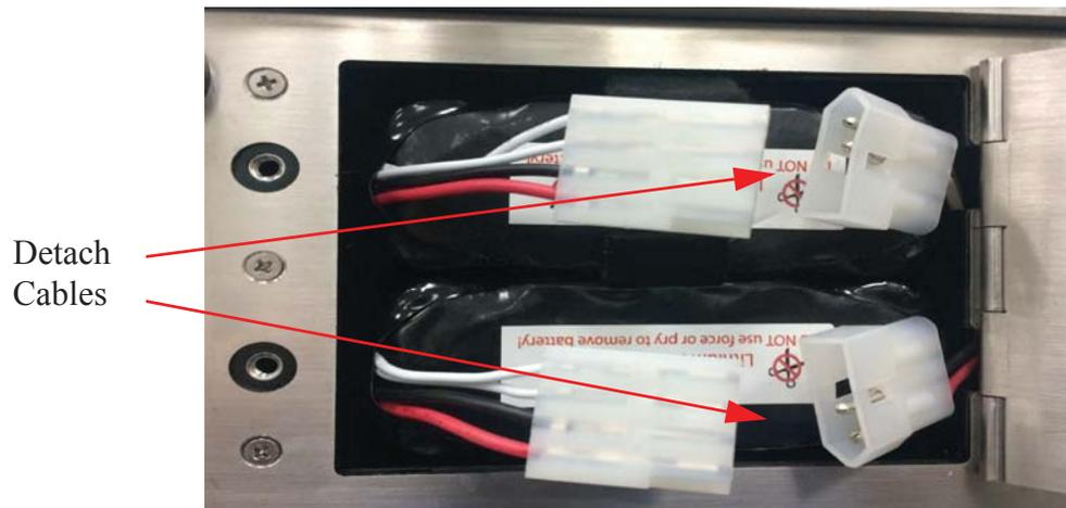
Figure 3-8 Removing Battery (Dual-Battery Units)
