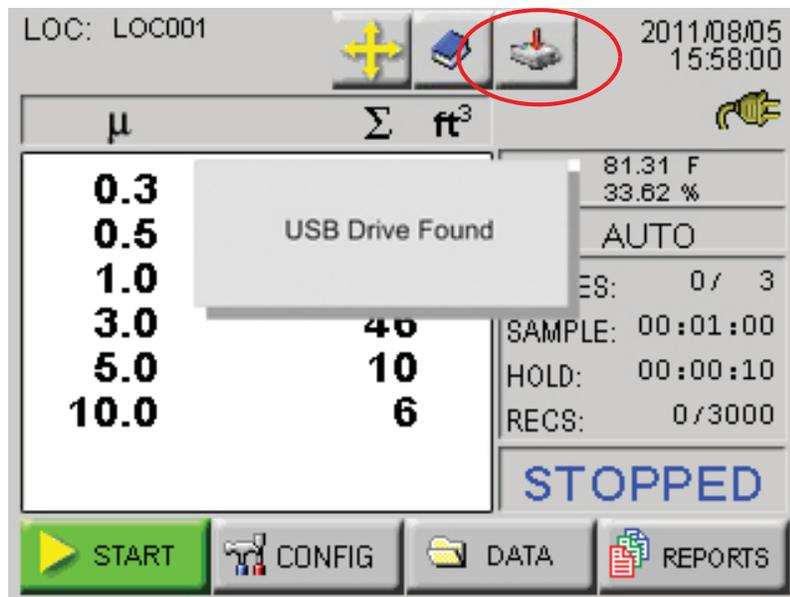
Figure 6-52 MAIN Screen, Flash Drive Attached, USB Mode
