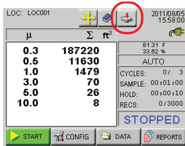
**Figure 5-4 MAIN Screen, Flash Drive Attached, USB Mode**
