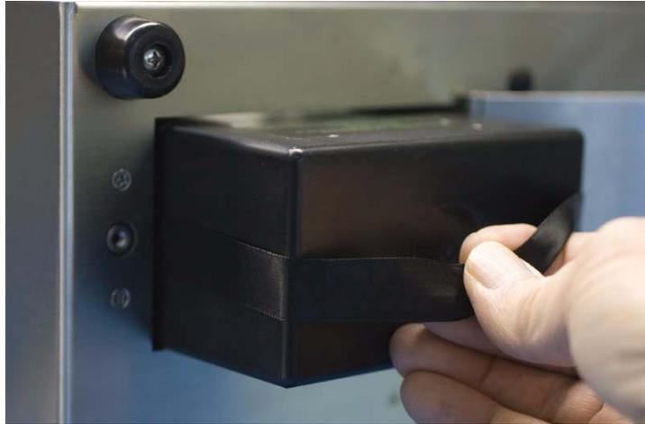
Figure 3-7 Removing Battery (Single-Battery Units)
