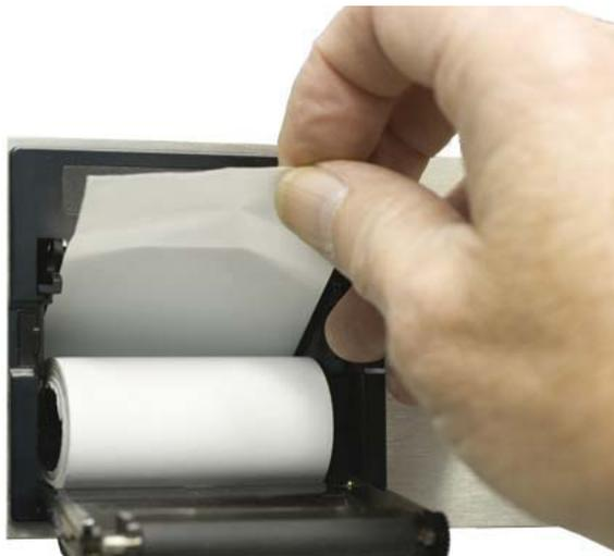
**Figure 3-12 Placing Paper Into the Printer**
