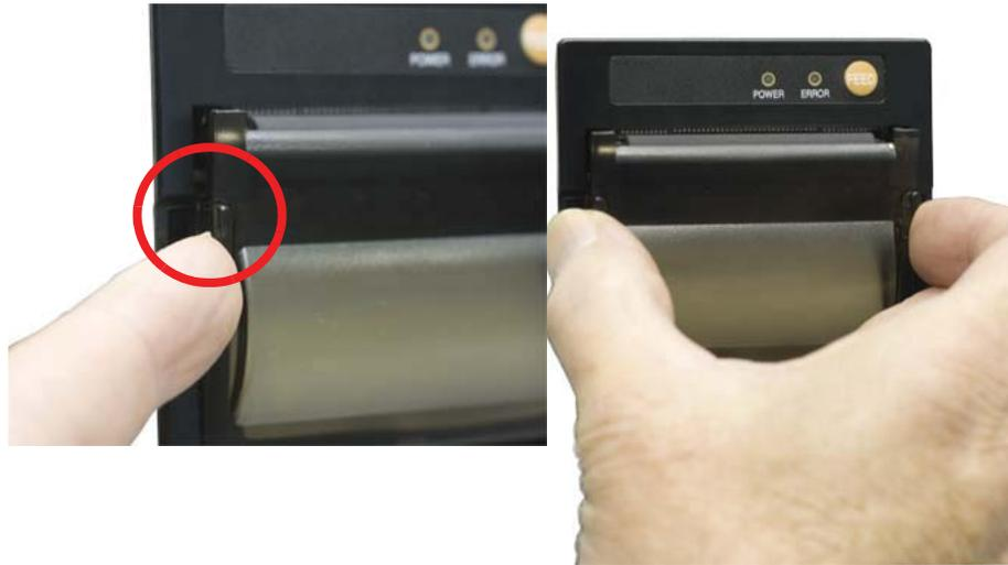
**Figure 3-11** Opening Printer Door
