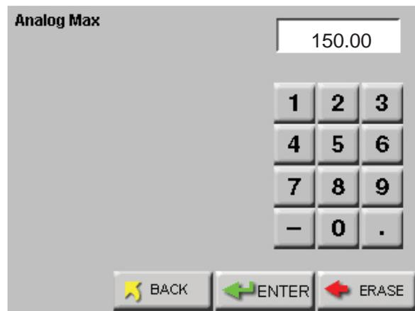
**Figure 6-24 Analog Min / Max Values Setting Screen**
