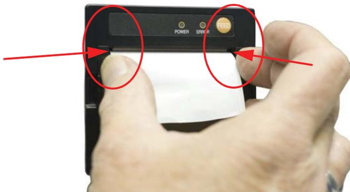
**Figure 3-13 Aligning the Paper**
