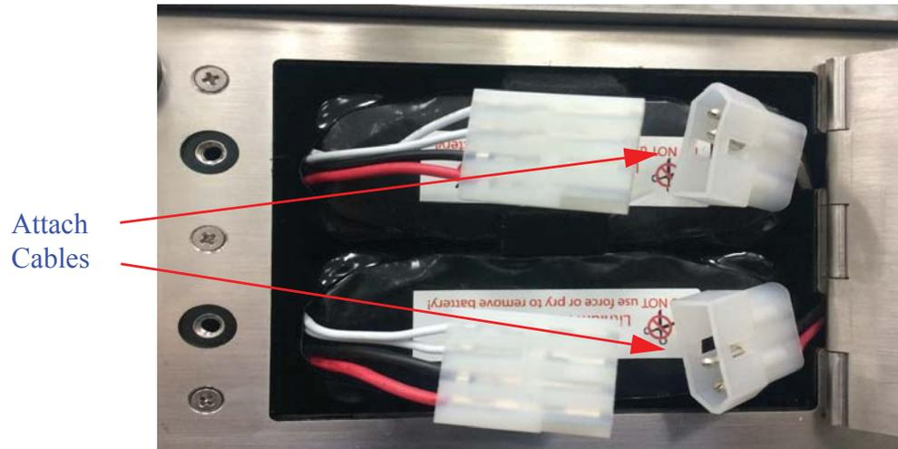
**Figure 3-6 Dual-Battery Compartment With Batteries**
