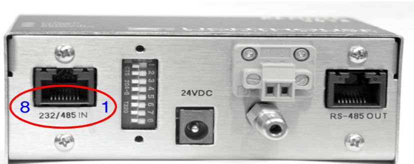
Figure 4-3 Communications Ports, Showing Pin Numbers
