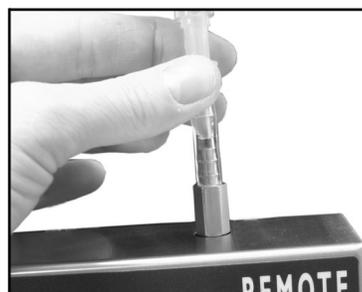
**Figure 3-7 Attach sample tubing to inlet**
