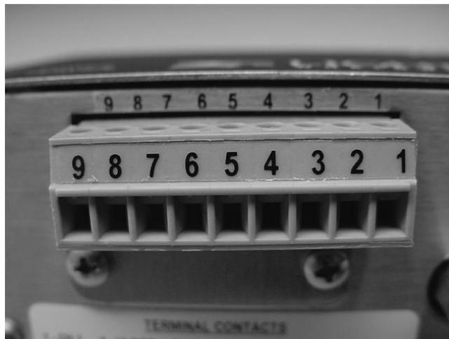
**Figure 3-9 J10 Connector With Plug Attached**
