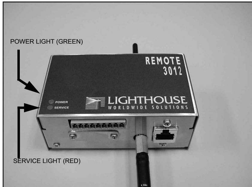
**Figure 3-1 Front Panel LEDs**
