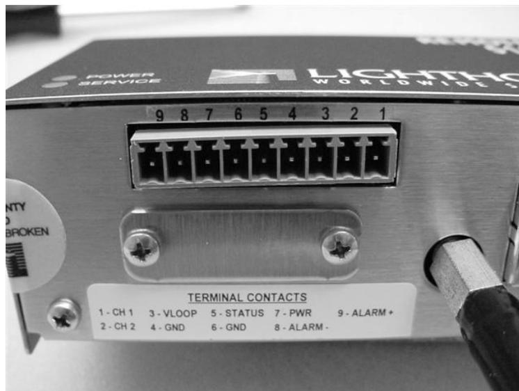
Figure 3-4 J10 Labeling (with Status feature on pin 5)
