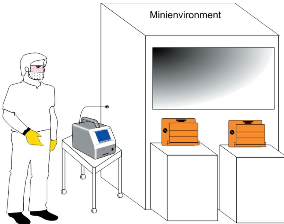
tuning process (see Figure 1). This generally is the same particle counter used to test and monitor the main cleanroom. Characterization is required to assure the tool is performing to the required cleanliness. Routine monitoring is also needed as an audit to assure that nothing has changed.
