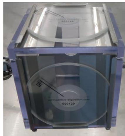
Figure 1: Box holder with witness plates as seen from the front
