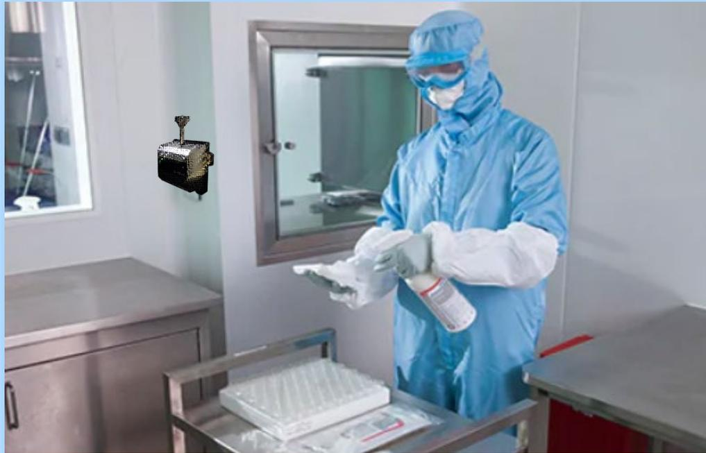
**When spraying cleaning solution near particle counters be careful to avoid the aerosol from entering the particle counter as the solution can deposit on the sensor optics and cause inaccurate particle count data and also fail the as found calibrations.**
