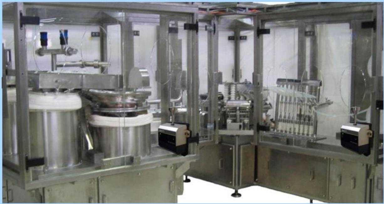
**Filling Machine being monitored with remote particle counters (with internal vacuum)**
