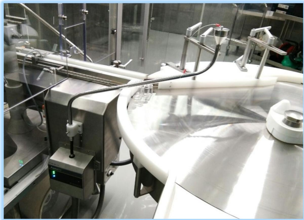
**1cfm Remote Particle Counter on filling line measuring 0.5 $\mu$ m and 5.0  $\mu$ m particle data**
