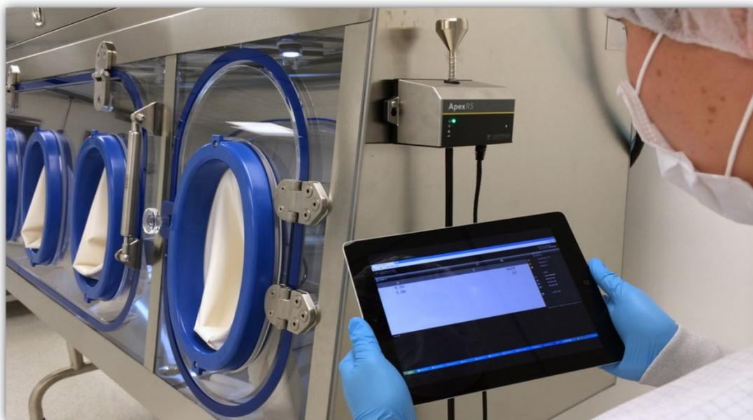
Fig 7 End User validation (PQ) of remote Particle Counter location in a Cleanroom – Grade B Environment.
