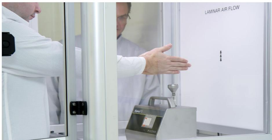
Fig.4 Study using a portable particle counter to validate sample probe placement and height inside LAF cabinet based on process manipulations
