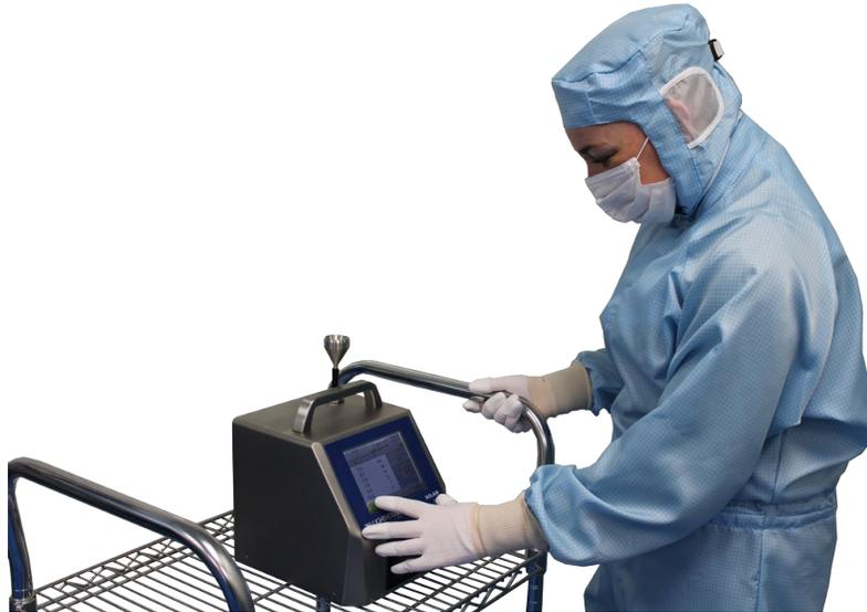
Operator setting up Particle Counter for Cleanroom Certification
