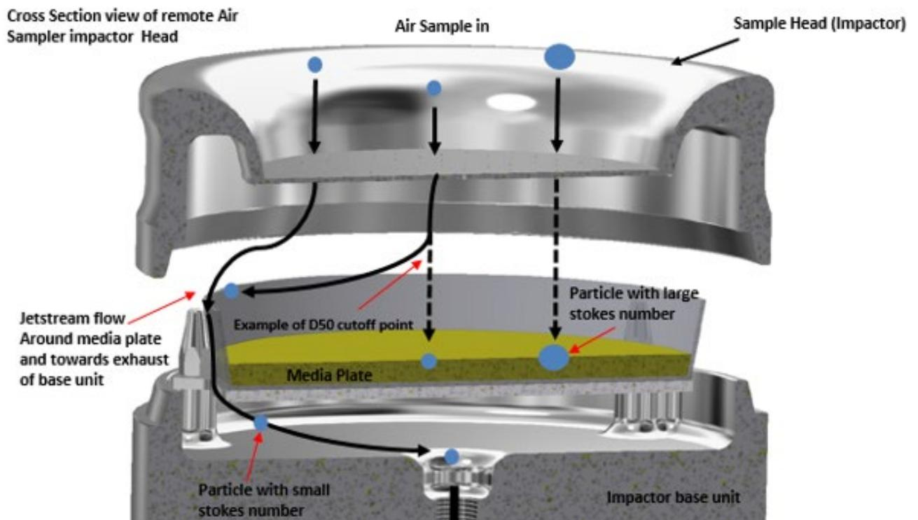
**Fig 3 Cross Section view of a Lighthouse Air Sampler Impactor**
