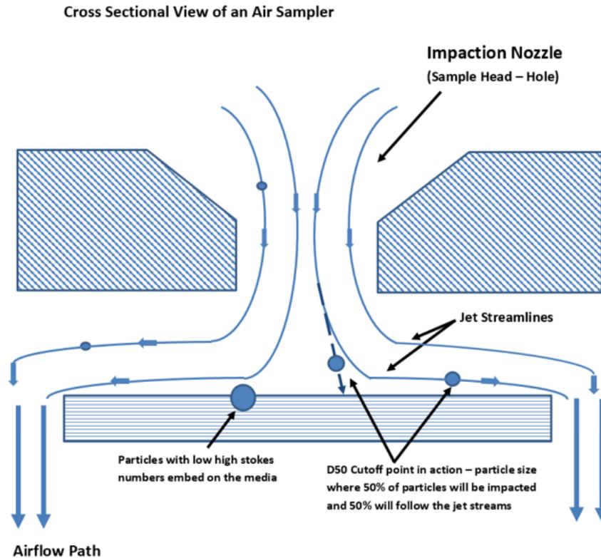
**Fig 2 Cross Section view of an Air Sampler Impactor**
