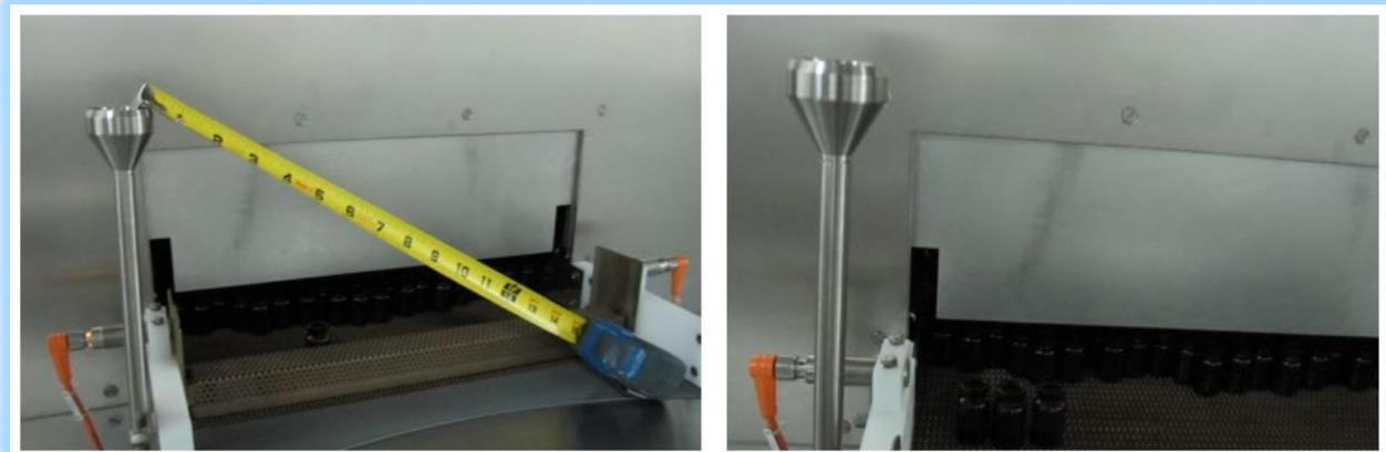
Example of ISP positioned within 12” of the process where sterile open vials exit a sterilization oven onto the fill line.
