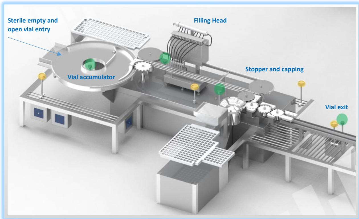
Example of a filling line with viable (orange) and non-viable particle counter (green) sampling locations based on a risk assessment with a scientific approach to capture events in critical locations.
