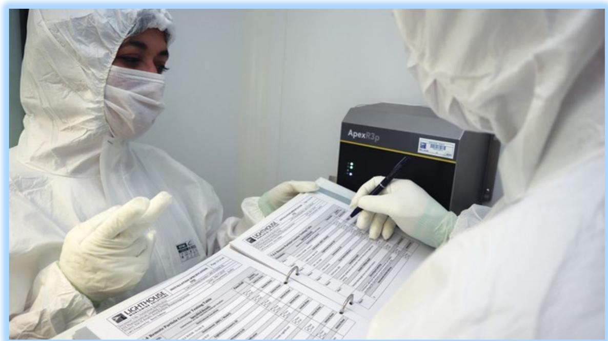
**Pharmaceutical Customer working with Lighthouse validation engineers conducting a PQ of a remote particle counter with internal pump in a Grade B cleanroom**
