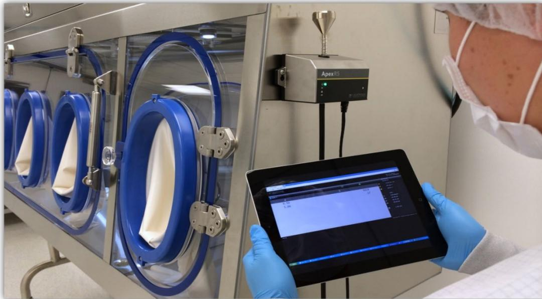
Cleanroom PQ Validation of Remote Particle Counter
