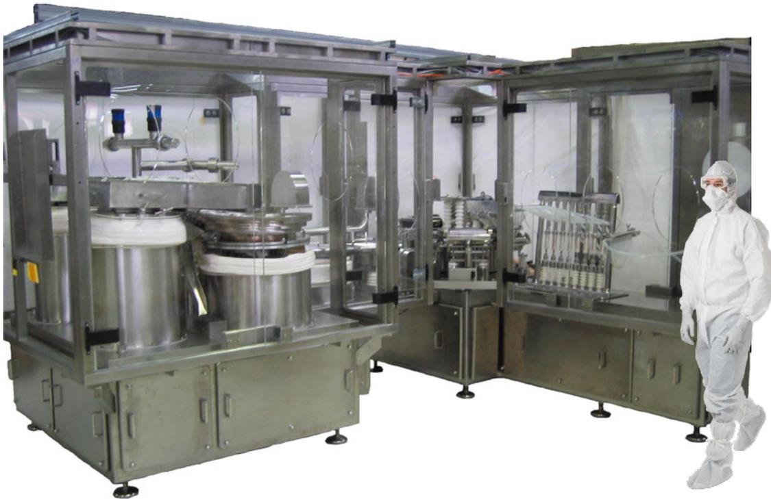
**Example of a Filling line for sterile injectable product fill**
