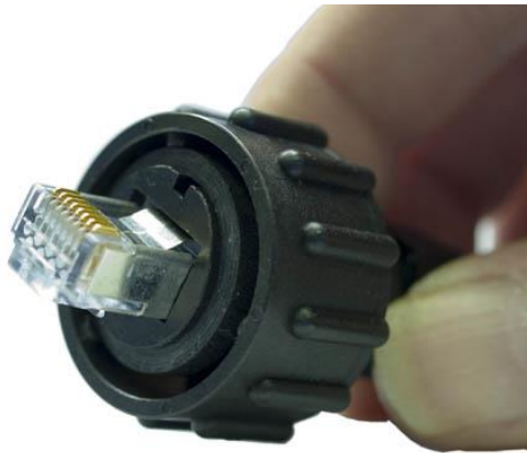
Figure 3-12 Cable Connector Completed
