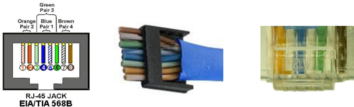
Figure 3-4 EIA/TIA-568B Color Code Example
