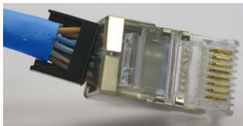
Figure 3-5 Loomed Wires Being Inserted into RJ45
