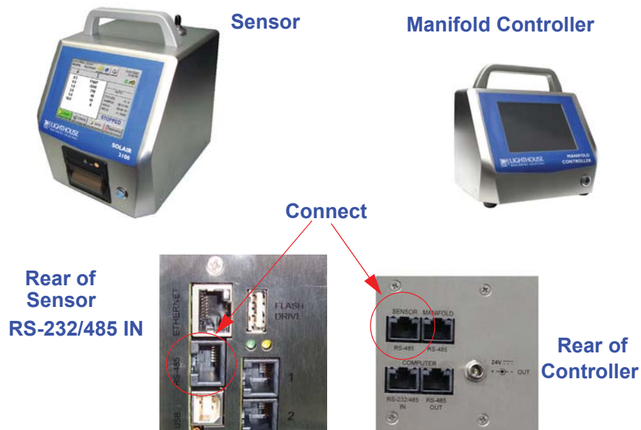
Figure 5-3 Connecting Sensor to Manifold Controller
