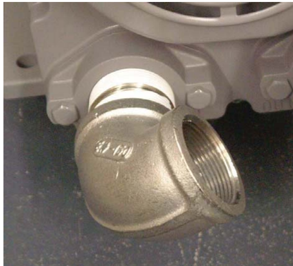
Figure 4-5 Pump's IN Port Elbow Installed
