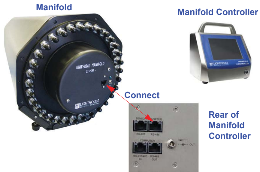
Figure 5-2 Connecting Manifold to Manifold Controller
