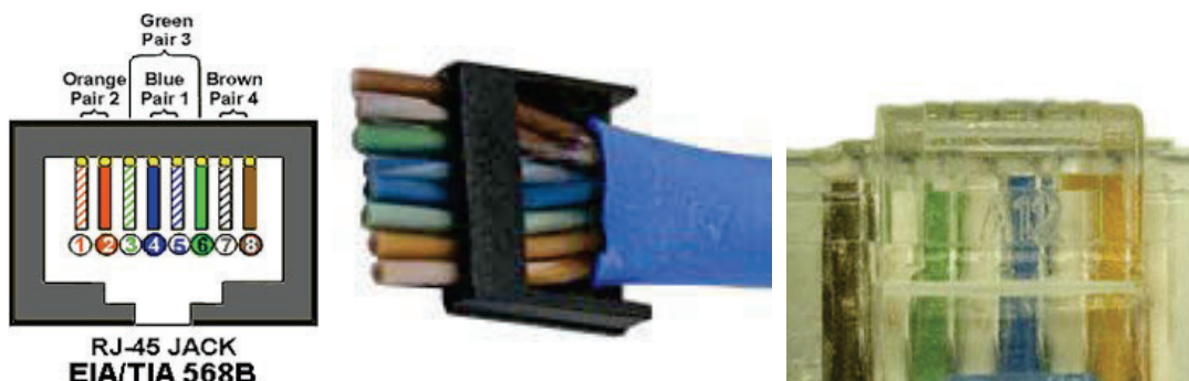
Figure 3-4 EIA/TIA-568B Color Code Example
