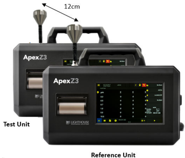
Baseline Setup 2 using portable particle counters
