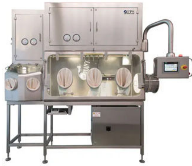
Fig.6 Aseptic Isolator with sealed gloved ports– Medium Risk
