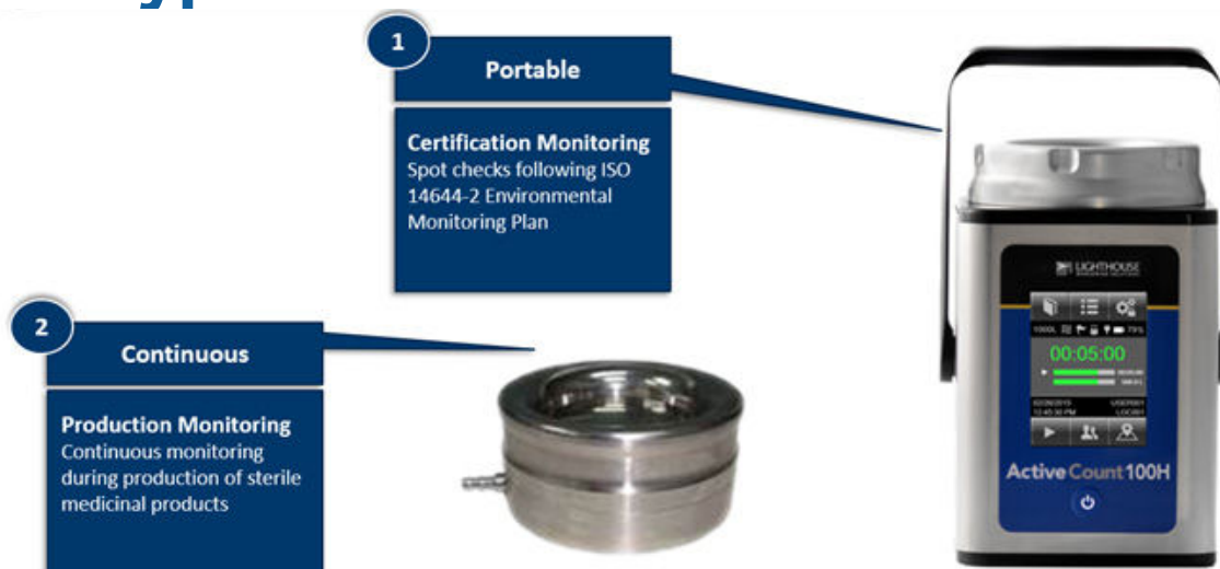
Fig. 9 Overview of two types of active air samplers 1.Portable 2.Remote
