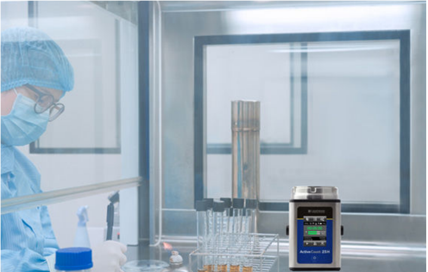
Fig.1 Biological Safety Cabinet testing using active air sampler with low flowrate.
