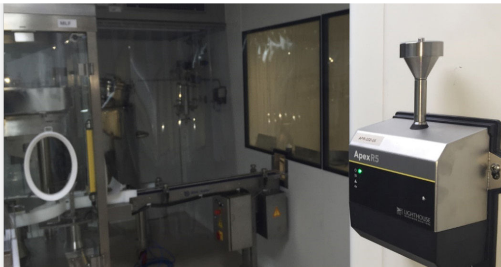
Remote Particle Counter in Grade B/ISO 7 Cleanroom
