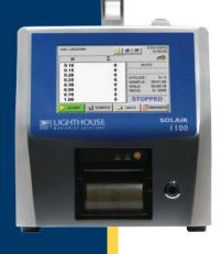
HE SOLAIR 1100LD leads the industry as the first-of-its-kind portable particle counter with 0.1-micron sensitivity and 1.0 CFM (28.3 LPM) flow rate using laser diode technology. Conventional HeNe (Helium Neon) particle counters require frequent cleaning and periodic laser tube replacement and suffer low concentration limits. The SOLAIR 1100LD is designed to operate in ISO class 1 to class 7 cleanrooms without concerns of it exceeding concentration limits.
