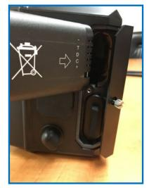
**Close the battery door.** Tighten down the battery door screw.
