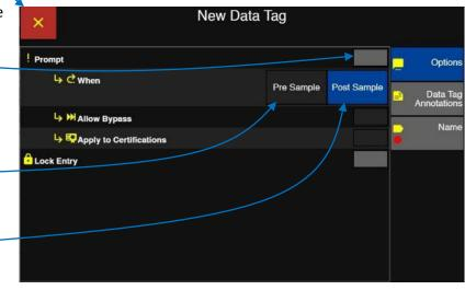
**Allow Bypass:** Enable this feature to allow the user to bypass entering the data tag prompt when it appears. User will be allowed to enter the data tag value later in the data record screen. *Note: Bypassing a data tag prompt will be noted in the Audit Trail.*
