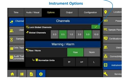
Global channels highlighted in green are ENABLED. Global channels highlighted in grey with strike through text are DISABLED. Press any green channel button and it will highlight grey with strike through text to indicate this channel has been disabled. Press any grey button and it will highlight green indicating it has been enabled.
