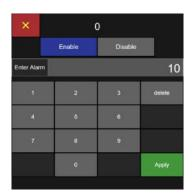
Press the Enable button and it will highlight blue indicating the Warning or Alarm has been enabled.
