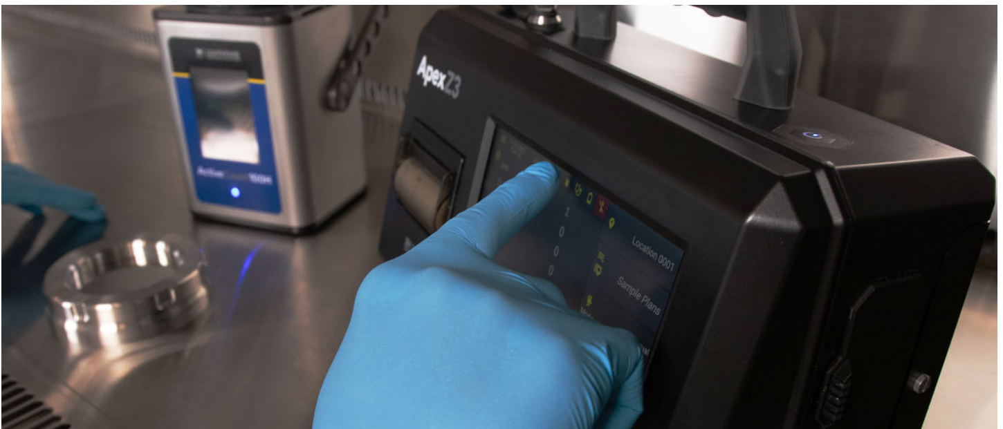
Compounding Technician setting up a Portable Particle Counter to monitor the compounding environment during compounding activities.
