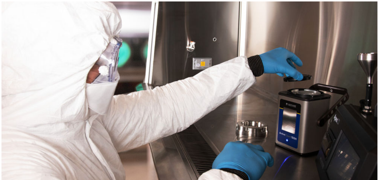
Compounding Technician setting up a portable Air Sampler to take samples prior to compounding activities inside a Biological Safety Cabinet (BSC).
