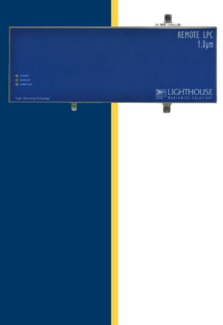
he Remote LPC LE has a range of 1.0 - 50 microns or 1.0 - 200 microns particle sizes in liquid. With a flow rate of 30 ml per minute. The sensor is designed to accurately measure up to 8 channels of simultaneous particle count data.
