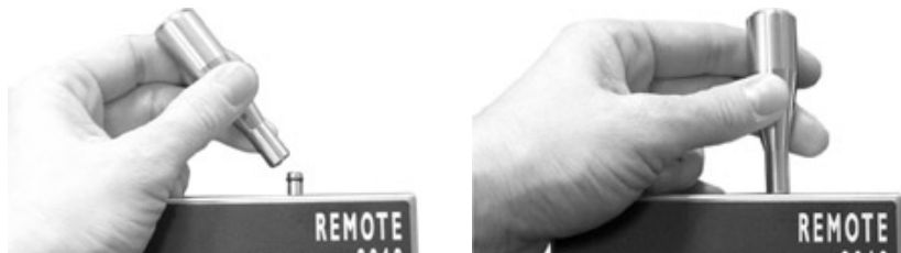
Figure 3-7 Installing probe directly on barb
