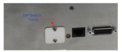
Figure 4-1 Panel Covering the DIP Switches
