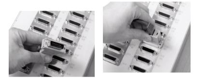
Figure 3-6 Connecting to SIU Frequency Port
