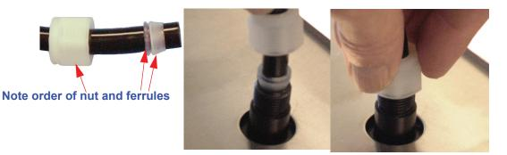
Figure 3-3 Attaching tubing with Ferrule and Nut Kit
