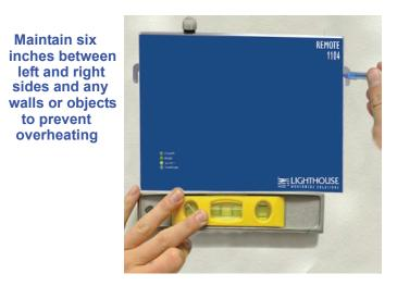
Figure 3-2 Marking Wall for Mount Point
