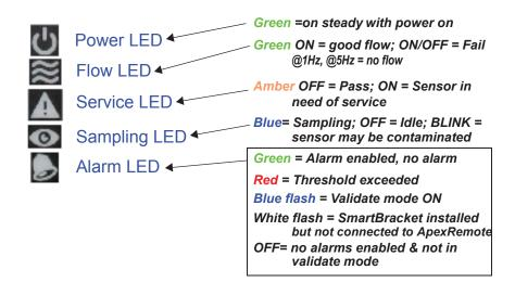
Figure 3-10 Front Panel LEDs
