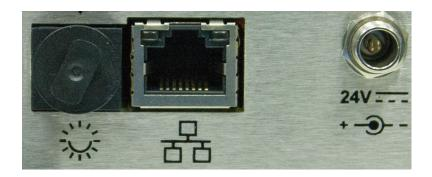
Figure 1-1 SmartPort, Ethernet and 24VDC Power Connectors
