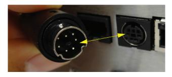
Figure 3-4 SmartPort cable into SmartPort
