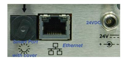
Figure 7-8 *PoE* Instrument Connections
