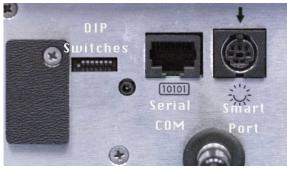
Figure 7-7 Serial Instrument Connections
