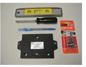
Figure 7-1 Required Tools and Hardware
