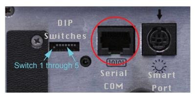
Figure 4-2 Serial COM Port
