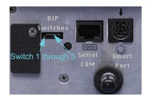
Figure 4-1 ApexRemote Serial Connectors and DIP Switch
