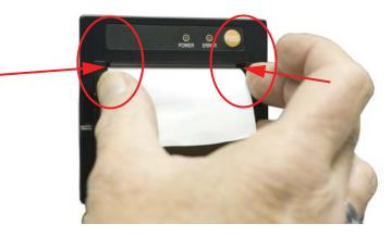
Figure 3-13 Aligning the Paper
