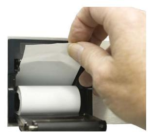
Figure 3-12 Placing Paper Into the Printer
