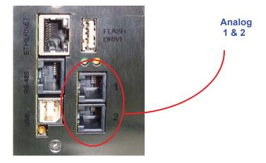
Figure 6-20 Analog Port Connectors
