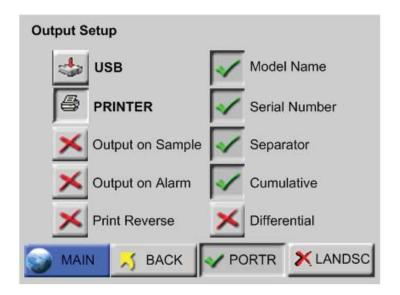
Figure 6-53 Output Setup Screen, Printer Settings
