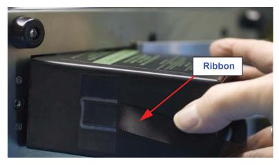
Figure 3-3 Inserting Battery
