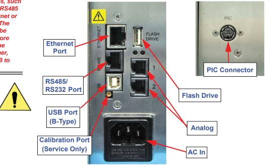
Figure 5-1 SOLAIR 3350, 5350 Rear Connectors
