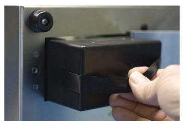
Figure 3-7 Removing Battery (Single-Battery Units)
