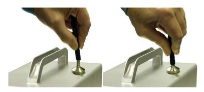
Figure 3-10 Installing Tubing Onto Inlet
