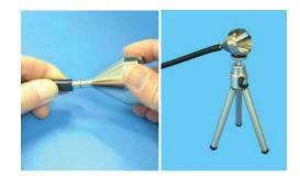
Figure 3-9 Tubing, Isokinetic Probe and Tripod
