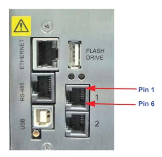
Figure 4-1 Analog Sensor Ports
