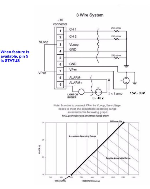
Figure 3-11 Application for a Three Wire System
