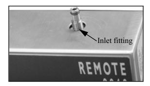
Figure 3-2 Connections on Top of Instrument
