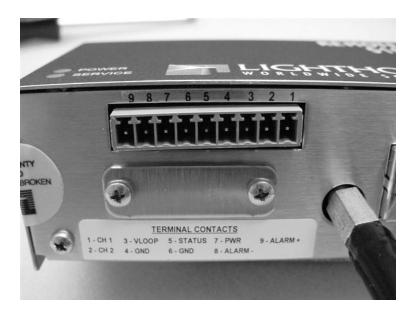
Figure 3-4 J10 Labeling (with Status feature on pin 5)
