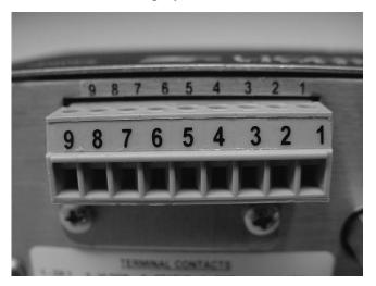
Figure 3-9 J10 Connector With Plug Attached
