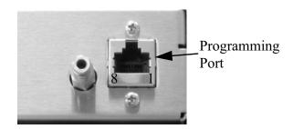
Figure 4-3 The Programming Port, Showing Pin Numbers
