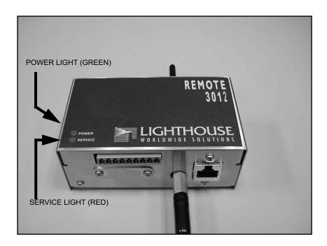
Figure 3-1 Front Panel LEDs
