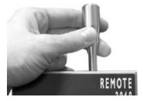
Figure 3-8 Installing Probe Directly on Barb
