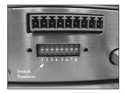
Figure 4-2 Panel Removed, Switches Exposed
