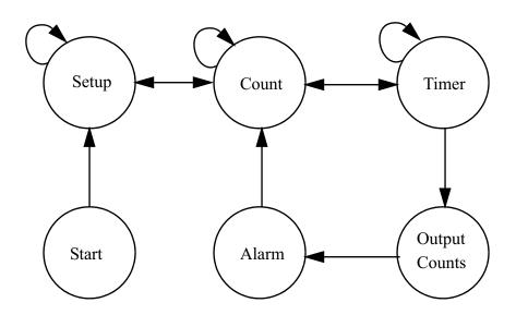
Figure 5-1 States for the 3012, 5012, 3102, 5102 Particle Counter
