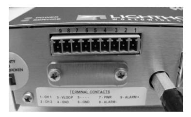
Figure 3-5 J10 Labeling (without Status feature on pin 5)
