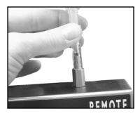
Figure 3-7 Attach sample tubing to inlet
