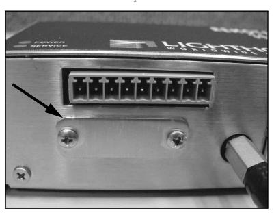
Figure 4-1 Panel Covering the DIP Switches
